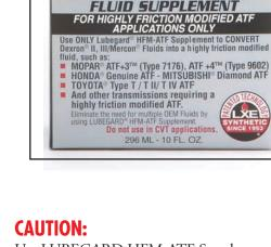
Use LUBEGARD HFM-ATF Supplement (Black Box) ONLY for applications that require highly friction modified fluids. Also do not use in CVT applications. Use in transmissions that do not have this requirement may cause excess wear and clutch slippage. Use LUBEGARD Automatic Transmission Fluid Protectant (Red Box - 60902) in all other ATF applications.
